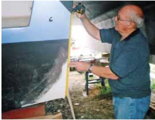
In one example the inboard hull depths were 500mm and 530mm respectively
