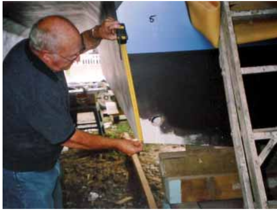
In one example the inboard hull depths were 500mm and 530mm respectively
