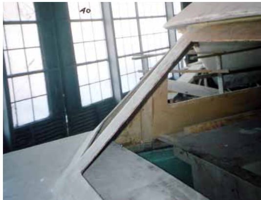
Stbd screen was 50mm and port screen 140mm out of wind
