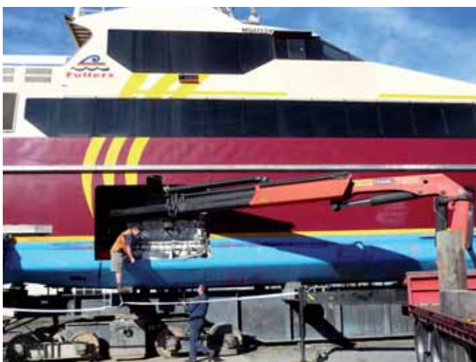
Removing the power plants
